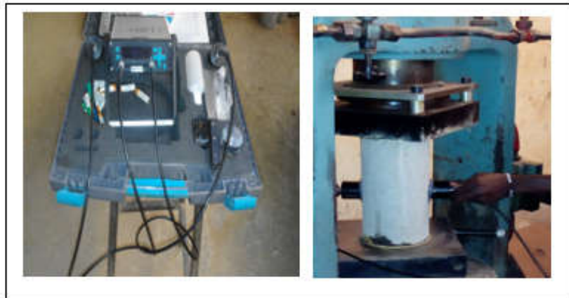
Fig. 3. Arrangement of transducers for pulse velocity measurement with Pundit-Lab
