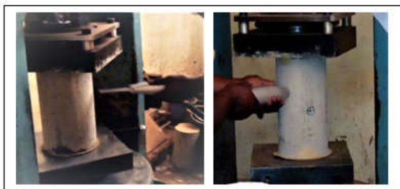
Fig. 5. Layout of the Schmidt model N standard hammer for rebound index measurements
