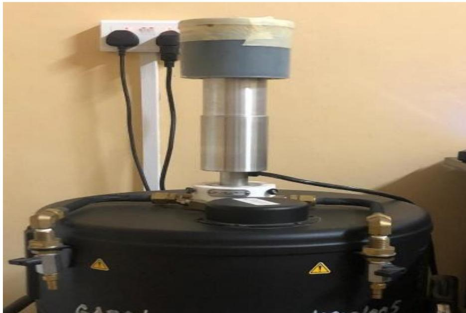
**Fig. 2. Detector-beaker installation**
