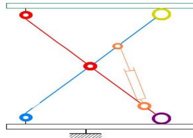
Fig. 5. 2D kinematic diagram of the lifting table
