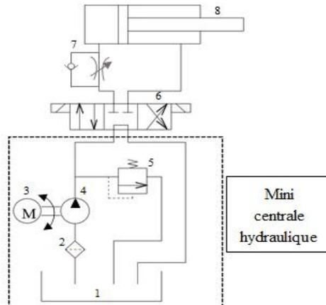
**Fig. 15. Hydraulic circuit of the lifting table**
