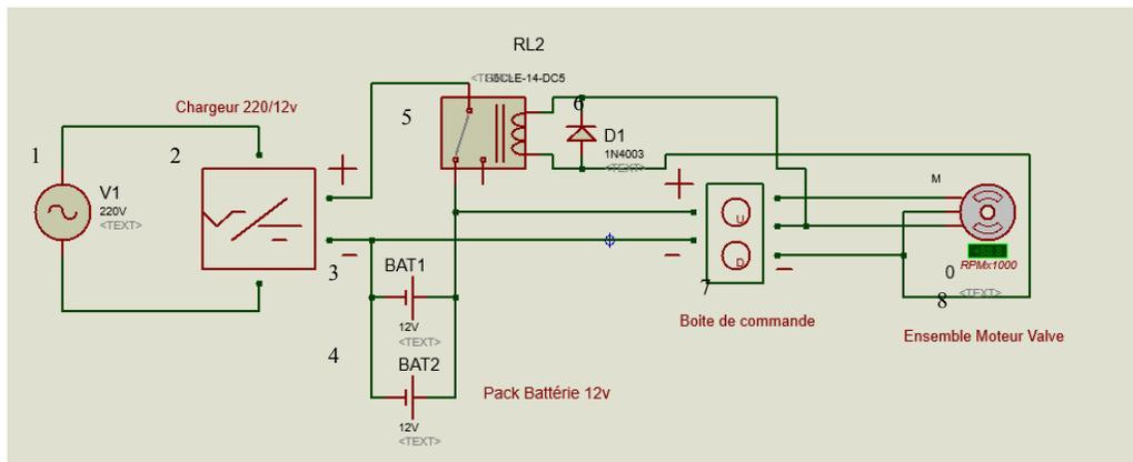
**Fig. 17. Electrical circuit of the lifting table**
