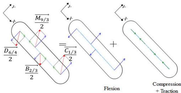
**Fig. 9. Stresses on the scissors**
