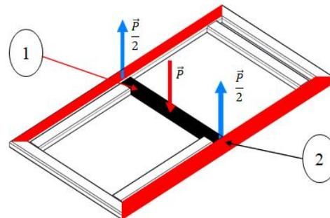
**Fig. 6. Forces applied to the platform structure**
